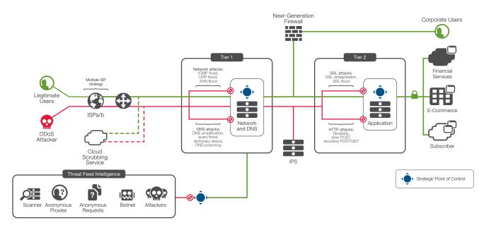
A two-tier DDoS protection architecture provides greater efficiency and flexibility in scaling security components.
